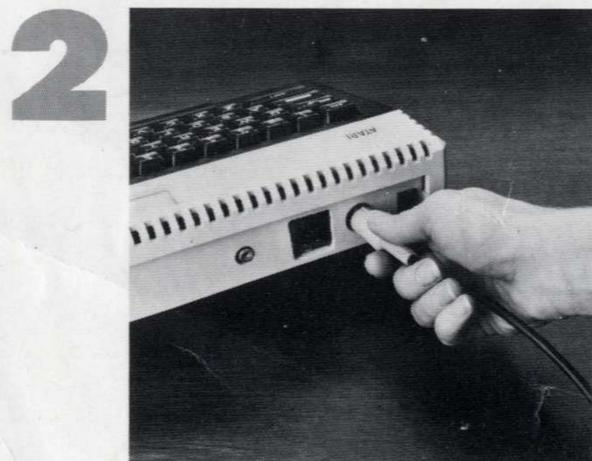
Plug the round connector of your power adaptor into the jack marked "POWER IN" on the back of your computer. Then plug the power adaptor into an electrical outlet.
