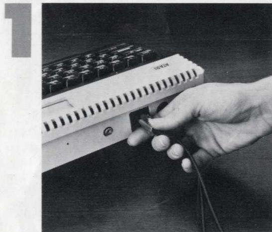
Attach the six-pronged plug of your cable to the jack marked "MONITOR" on the back of your computer. Connect the other end of the cable to your television or monitor according to the instructions provided with your set.
