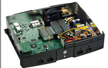
An opened first-generation Xbox console with the hard disc drive and optical drive removed, showing components like the power supply (far right), cooling fins, cooling fan, and case features
