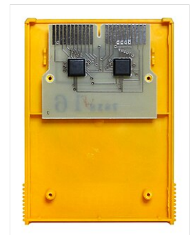
An opened Fairchild Channel F ROM cartridge, illustrating the ROM chips mounted to a circuit board within the casing. The cartridges were inserted into the console via the exposed contacts on the top of the board.
