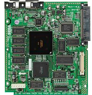
The Sega Dreamcast motherboard, incorporating more complex IC circuitry
