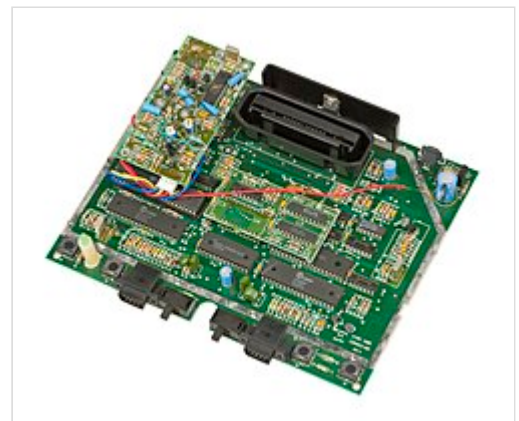
European motherboard modified by Atari to output RGB through a SCART connector
