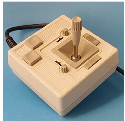
CH Products Mach II analog joystick for Apple II computers. The small knobs are for (mechanical) calibration, and the sliders engage the self-centering springs.
