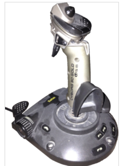
Saitek's Cyborg 3D Gold around the 2000s. Note its throttle, its extra buttons, and its hat switch.
