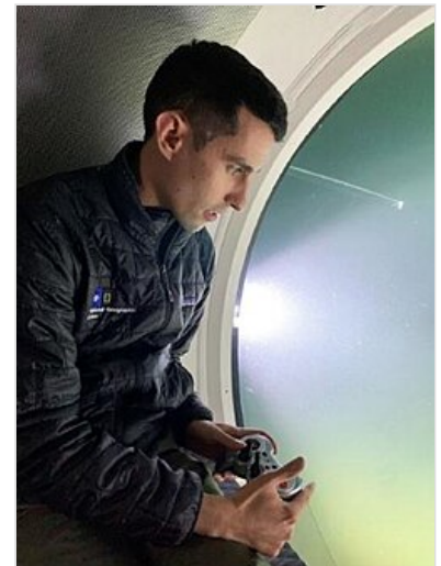
Trent Tresch piloting the OceanGate Cyclops 1 submersible using a modified Logitech F710 Game Controller
