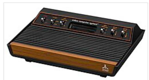
The second VCS model has lighter plastic molding and shielding, and a more angular shape, than the 1977 launch model.
