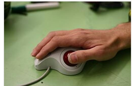
Logitech TrackMan Marble Wheel designed to use the ball with the thumb
