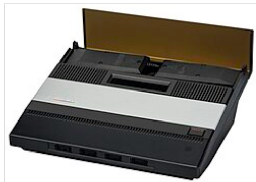
The 5200's large size is due in part to controller storage in the back of the unit.
