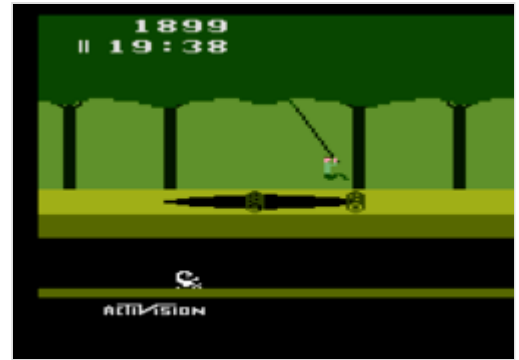
Pitfall! (1982) has more advanced graphics than the games the VCS launched with. The black bar on the left provides extra time for the program to prepare graphics between each scanline. [71]
