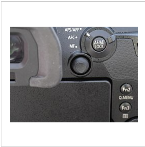
Miniature joystick to be operated by the right thumb, next to an electronic viewfinder
