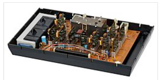
The inside of the Magnavox Odyssey showing its motherboard and battery compartment
