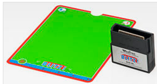
Games came supplied with color overlay sheets to compensate for the limitations of the screen.
