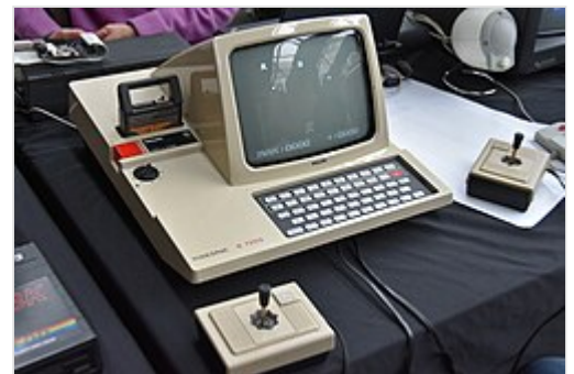
The Videopac G7200, unlike Videopac G7000, had a 9" (23 cm) black & white display built in.
